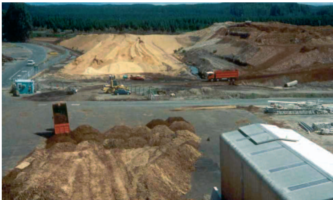
Mixing by the loader operator of the plant conveyor maintains the optimum feedstock moisture content to match the combustion system design.
