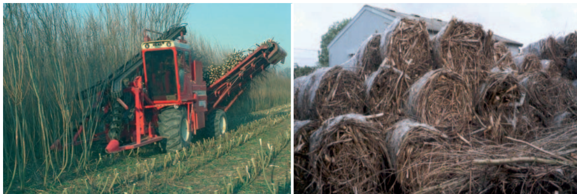
Equipment designed and manufactured to harvest new crops coppiced Salix, and store the biomass, (here shown as round bales of Salix stems) are relatively expensive in terms of USD/t harvested due to lack of mass production and limited demand.
