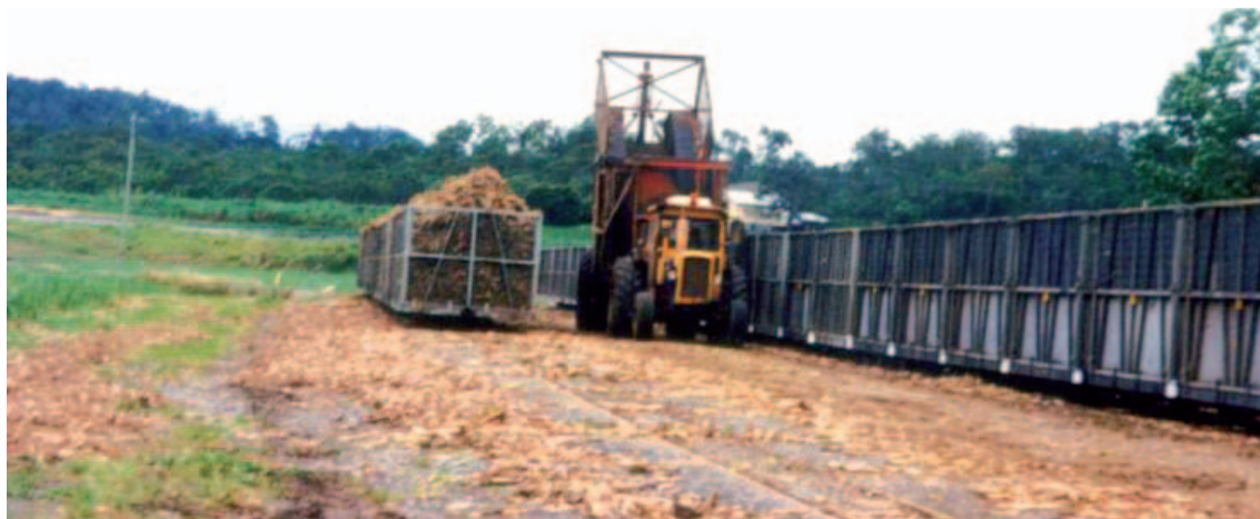
A tractor high-rise tipping trailer used to collect billets by running alongside a sugarcane harvester then transferring the load to bins on a mini-rail transport system for delivery to the sugar mill.
