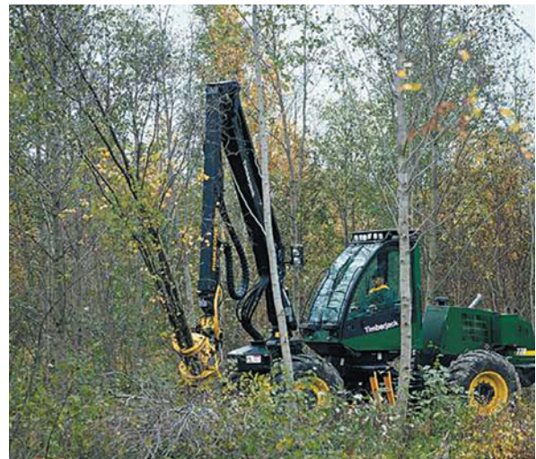
Mechanised harvesting of small trees for biofuel (Courtesy Dr Arto Timperi, Timberjack)
