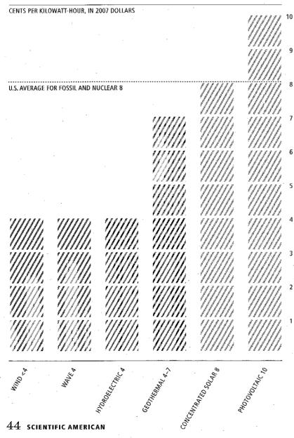
in 2007 of conventional power generation and transmission was about 7¢/kWh, and it is projected to be 8¢/kWh in 2020. Power from wind turbines, for example, already costs about the same or less than it does from a new coal or natural gas plant, and in the future wind power is expected to be the least costly of all options. The competitive cost of wind has made it the second-largest source of new electric power generation in the U.S. for the past three years, behind natural gas and ahead of coal.
