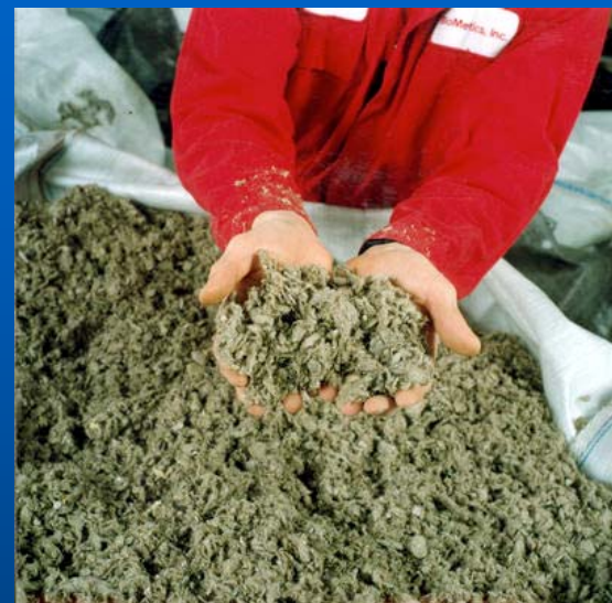
Photo Source Above: NREL. Dried paper mill sludge is used as feedstock in the demonstration facility of a Biofine pilot plant in South Glens Falls, NY
